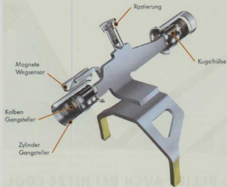
Bild 4: Schaltaktorik am Beispiel Schaltgabel 1./3. Gang Figure 4: Gearshift actuator system using the selector fork for 1st/3rd gear as an example
